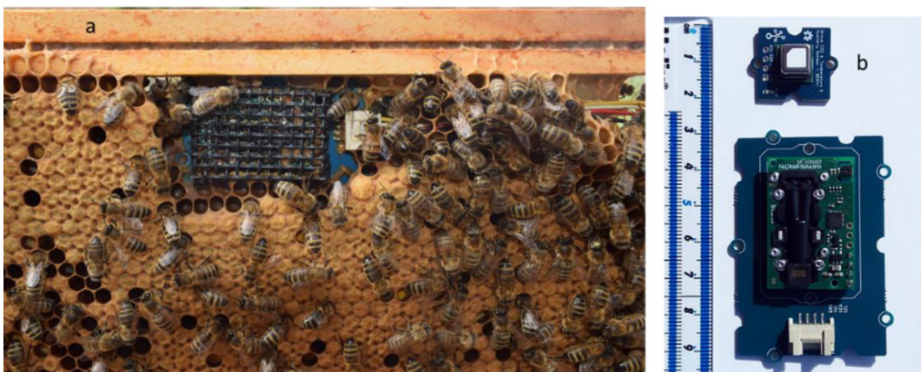
Figure 2.1. (a) SCD30 installed in brood box frame showing propolis coating on the protective mesh. (b) SCD30 (lower) and SCD41 (upper) sensors with a ruler to show the relative sizes of the two devices. © Martin Bencsik
