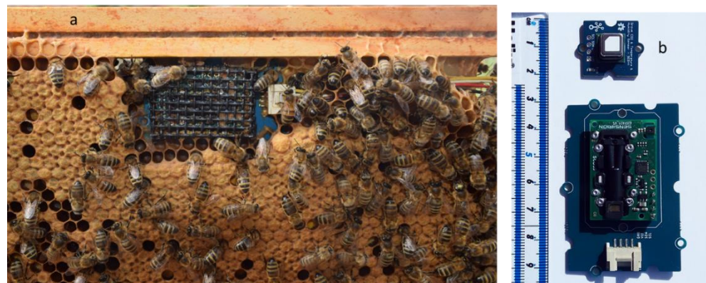
Figure 1. (a) SCD30 installed in brood box frame showing propolis coating on the protective mesh. (b) SCD30 (lower) and SCD41 (upper) sensors with a rule to show the relative sizes of the two devices.
